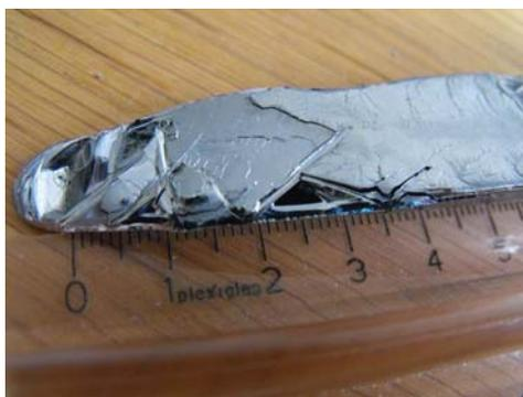
**Figure 1.** SnSe ingot as synthesized extracted from the quartz vial. The strong tendency to crystal growth is visible at the surface of the sample.
